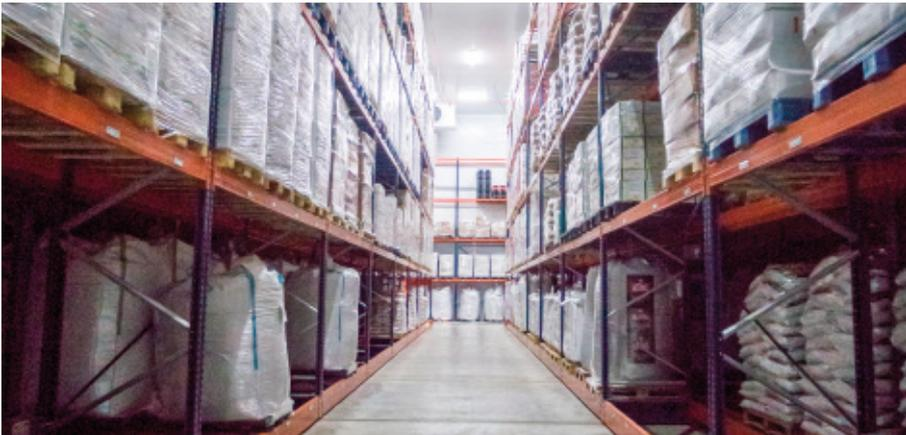
Mecalux has equipped the three frozen storage chambers of Frío Valencia with Movirack mobile pallet racking. This system makes full use of the available surface area to provide a storage capacity of more than 7,700 pallets and, likewise, to offer direct access to the SKUs the moment a work aisle opens.
