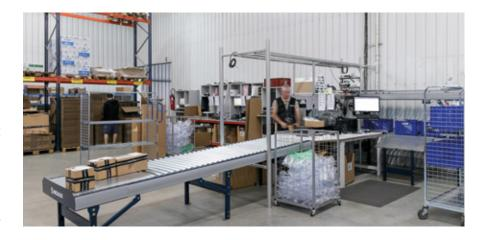
The circuit is adapted to the demands of the centre and incorporates straight sections, curves and a ramp with conveyor bands to move the boxes at a controlled speed from the upper floor to the lower warehouse
