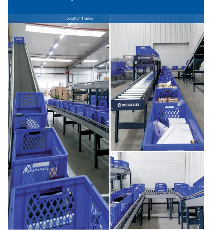
Algam, distributor of musical material and audio equipment, has automated the order consolidation area of its warehouse in Thouaré-sur-Loire (France). There, customer orders are verified and conditioned before their subsequent shipment. Mecalux has installed a box conveyor circuit that links the warehouse with this fully automated area.
