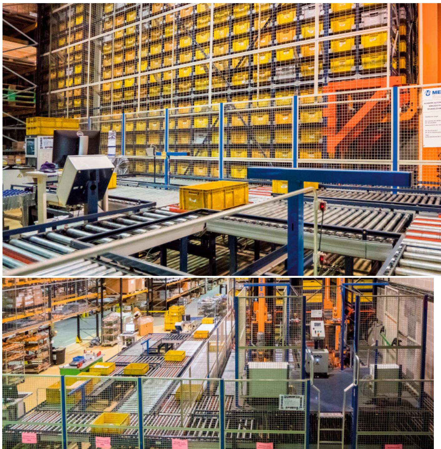
Two U-shaped picking stations are set up perpendicular to the main circuit. Picking is done via the "product-to-person" principle, in other words, the stacker cranes provide the merchandise to the operators automatically. The operators then extract the items indicated on a screen by the system and deposit them into the corresponding order.
