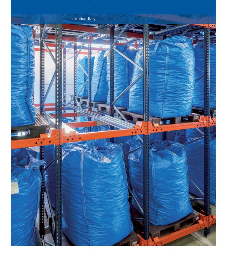
The cork manufacturer Belbo Sugheri has installed push-back racks from Mecalux in its storage facility located in Calamandrana (Italy). These racks, able to house up to 264 pallets, have multiplied the number of stored pallets, as well as accelerated its loading and unloading process.
