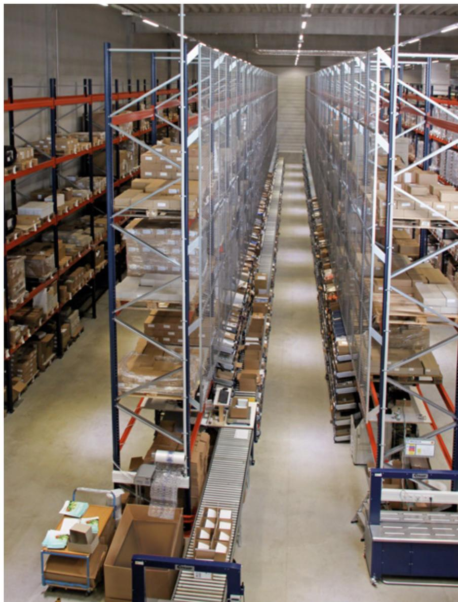
Attached to the racks, a free rolling, non-motorised conveyor acts as a prep table so that operators move boxes manually to the most suitable position. Operators collect products from the racks that run down both sides and place the items inside the order box.
