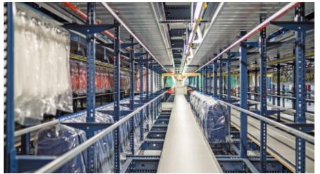
The tubes used for hanging garments on the racks are located at an optimum height from an ergonomic point of view and, although they have bearings every 2.2 m, the hangers slide and are grouped by items without producing any kind of interference.
