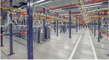
Spaces between pedestrian aisles are protected to avoid garments falling from one floor to another
