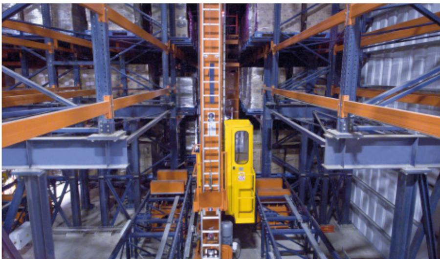
When working with perimetral type pallets (with open skids on all four sides), perpendicular cross ties were placed on the rack beams to support the pallets and thus ensure the stacker cranes handles them safely. This type of pallet improves stability during refitting.
