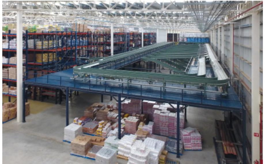
an intermediate walkway; three for picking and two for reserves. To prepare orders, operators deposit SKUs on a conveyor circuit that crosses through the central part of the different picking floors.
