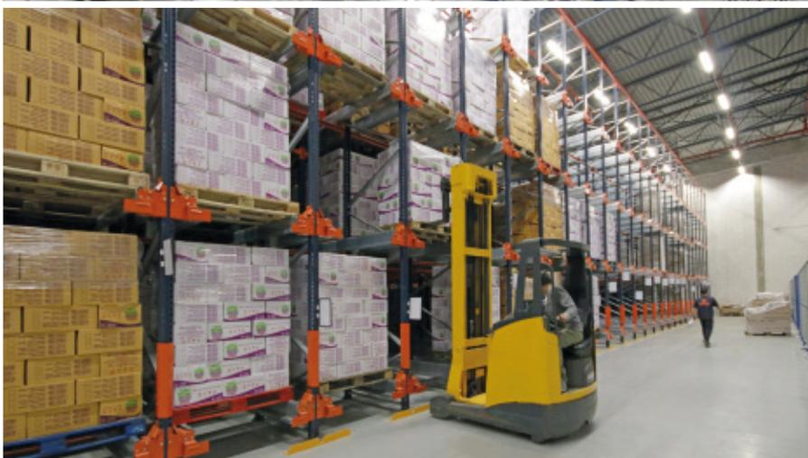
Firat Food, a food and beverage wholesaler, has reorganised operations in its French warehouse to streamline picking. Mecalux supplied pallet racking, the high-density Pallet Shuttle system and a roller conveyor, which joins the different areas that make up the installation.
