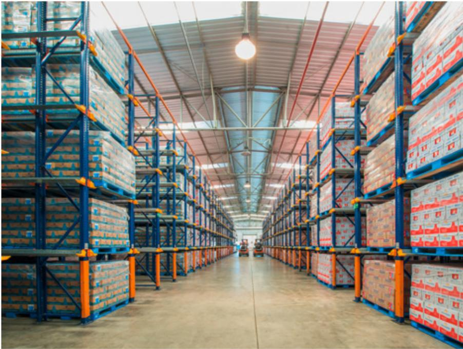
Operators, aided by reach truck, enter the inner lanes with the load perched above the level where it must be deposited. Both loading and unloading of the goods is performed in the same aisle, but in reverse.
