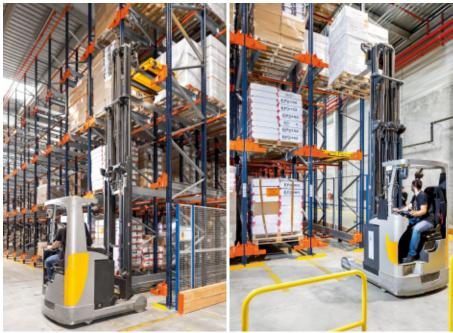
A total of 116 channels, 9.5 m in depth, offers a storage capacity of more than 1,200 pallets of 800 x 1,200 mm
