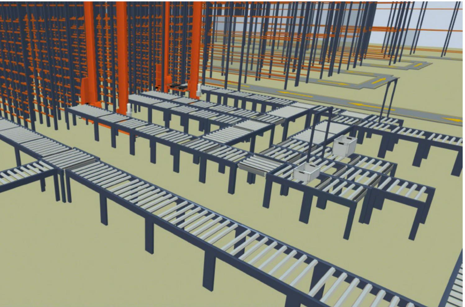
Galileo receives commands from the WMS, then sends the corresponding signals to the automated warehouse for boxes and helps pallets move to their destination
