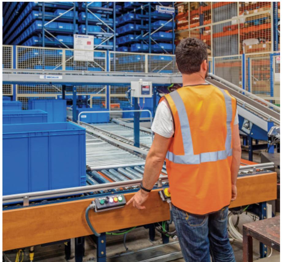
The frontal part of the warehouse is where a roller conveyor circuit is installed, which takes goods to the two picking stations. These comprise an order prep table with enough space to work with waves of four orders at a time. Next, the operators collect the products instructed by the WMS and place these in the correct box that will be sent to the consolidation area, located on one side of the warehouse. There is also a replenishment post located alongside the picking stations.
