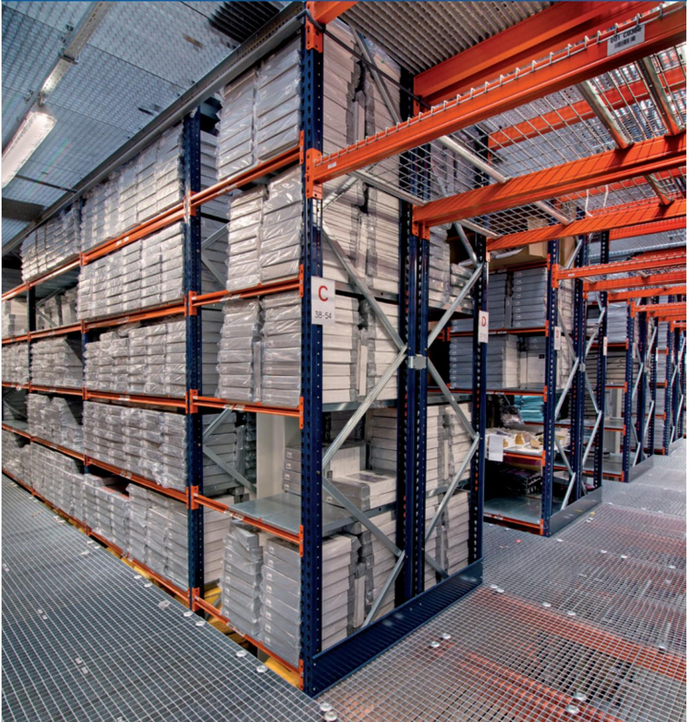
Mecalux has supplied all the storage systems in the new Eurofirany warehouse in Żywiec (Poland). On one side, there is a total of three floors of racks with walkways and on the other, cantilever racks for longer articles. The objective of both solutions is to classify goods according to their size and demand, as well as to streamline storage and picking tasks.
