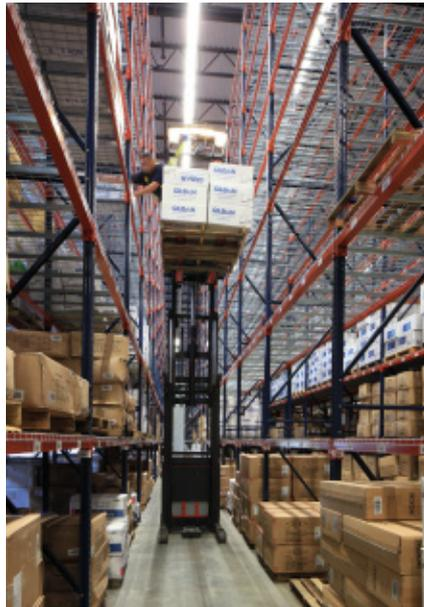
The result is a storage solution with almost 12 m high pallet racks set up to store both pallets and boxes on mesh shelves.
