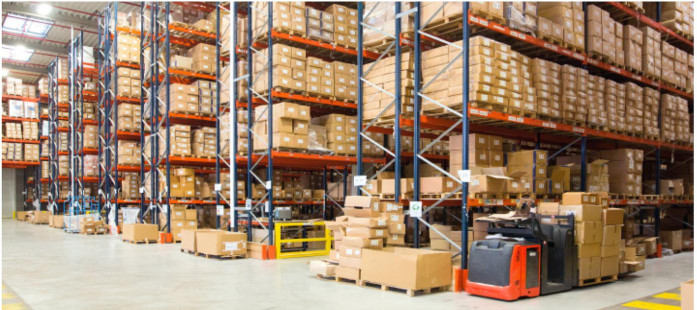
Due to this large variety of pallets, the racking levels were adjusted to the goods being stored and to its operations. Picking is done directly off the pallet in the lower rack levels, leaving product reserves on upper levels.
