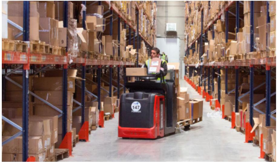
To pick items located on the first few levels, the operators use order pickers that raise to an appropriate height.
