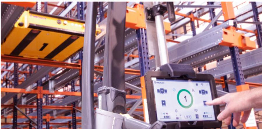
Storage processes are tablet run, through which orders are sent to the Pallet Shuttles. They have a touch-screen interface and a very intuitive software that requires no special training to use.
