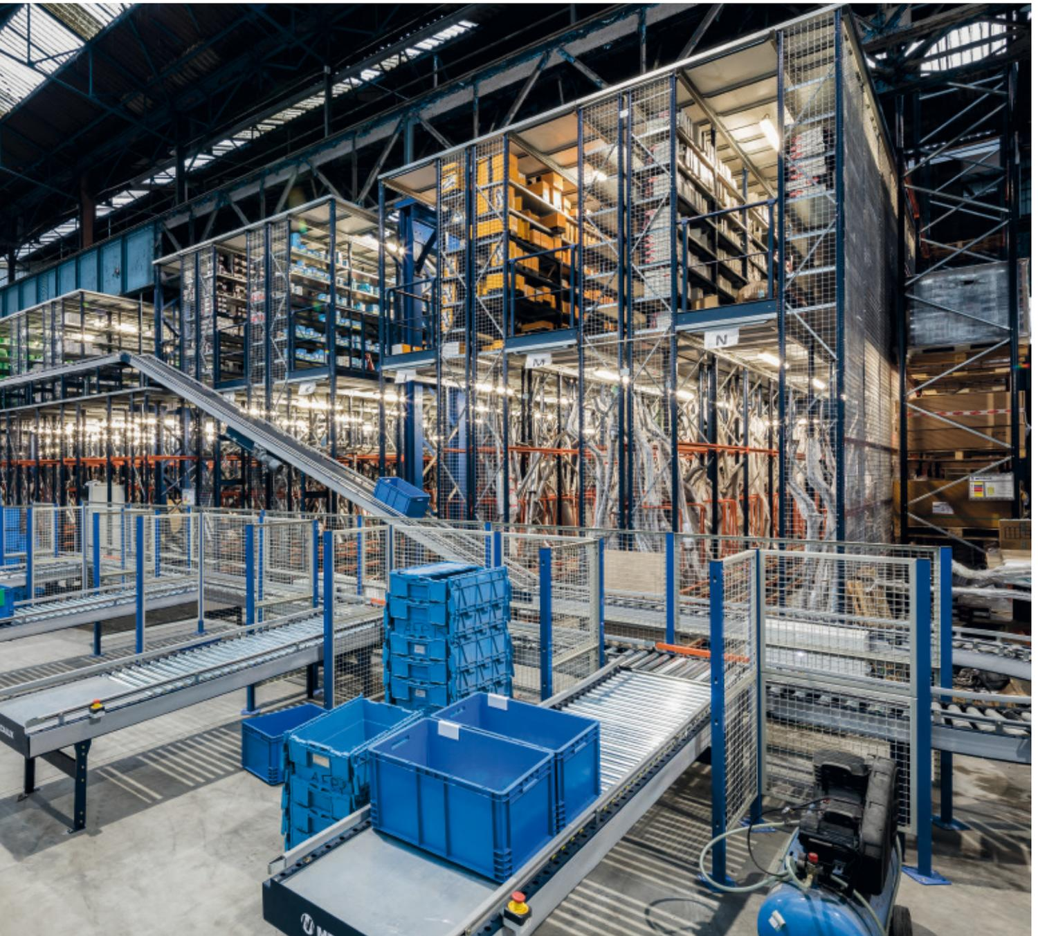
Racks with walkways take full advantage of the height of the distribution centre to max out available space and provide greater storage capacity
