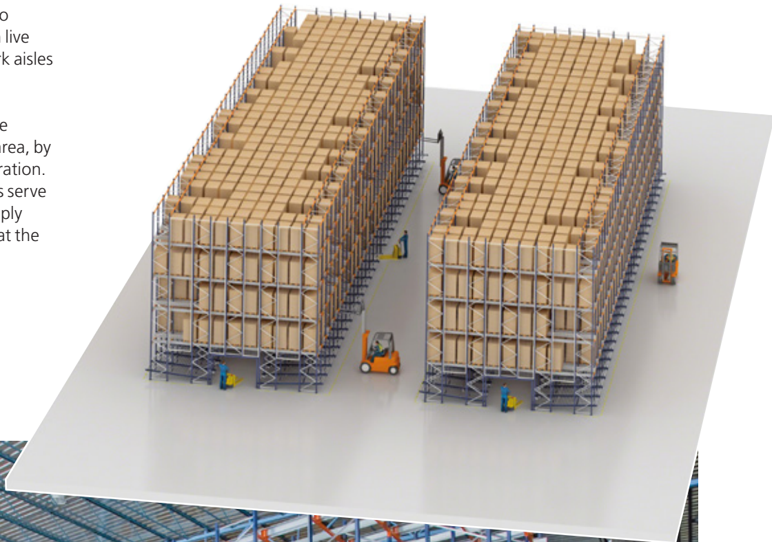
Solution 4. A warehouse with the semi-automated Pallet Shuttle system with two blocks combined with live levels for picking.
