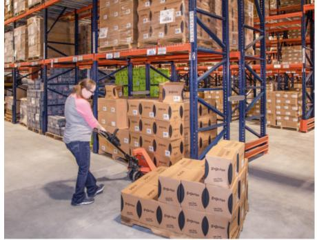
The result is a new 25,000 m<sup>2</sup> distribution centre, 75% of which is covered by 14 pallet rack aisles that are 8.2 m high and 12.8 m long. The storage capacity now stands at 3,908 pallets that measure 1,000 x 1,200 mm (GMA or perimeter pallet) with a 1,000 kg maximum unit weight.
