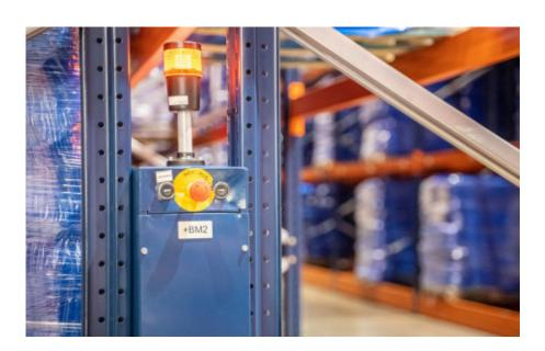
"We were particularly impressed by the quality and smooth operation of the racks," says Xavier Roca. To open the working aisle, the operator gives the command by means of a radio remote control unit.
