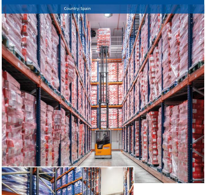
Mecalux has equipped the two new frozen storage units at Càrniques de Juià and Càrniques Celrà (companies that are part of the Olot Meats Group) in Girona (Spain) with Movirack Mobile Pallet Racking. This highdensity system is ideal for frozen storage units. Its advantages: making the most of the available surface area and reducing energy consumption per pallet by optimising storage unit volume. In total, the two warehouses manage more than 19,500 pallets.
