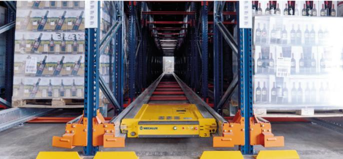
The Italian logistics operator Genta S.n.c. has a modern distribution centre made up of compact racks with the Pallet Shuttle system and pallet racks from Mecalux. The resulting storage capacity exceeds 7,000 pallets with alcoholic beverages. Space optimisation and fast product inputs and outputs ensure quick deliveries to customers worldwide.
