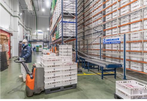
Automation not only has boosted the throughput of the warehouse, but has also been key for maintaining the cold chain necessary for properly preserving the meat. As for the safety of the workers and of the facility in general, the installation was equipped with automatic fire doors. If activated, the warehouse would be hermetically sealed to prevent the spread of flames and to allow for rapid evacuation of personnel.
