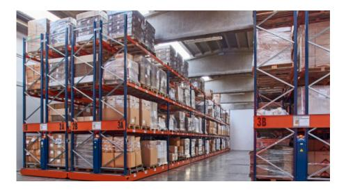
level-high lanes. This solution reduces the number of aisles in the interest of maximising space and, as a result, increases storage space.
