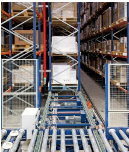
The installation at Industrias Cosmic in Caldes de Montbui, Barcelona, consists of an automated warehouse with live channels and a picking station at the front, plus a warehouse with adjustable pallet racking for bulkier products. The project included the Mecalux Easy WMS warehouse management system, responsible for managing all the activities carried out at the site.
