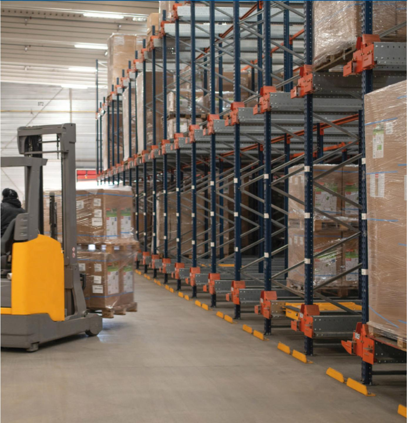
French company Trigano Jardin has opened a new distribution centre in the village of Cormenon (France) with racks served by the Pallet Shuttle system. This solution has provided the company with two advantages: optimal use of the surface area to achieve maximum storage capacity (up to 3,397 pallets), and constant, error-free inflows and outflows.
