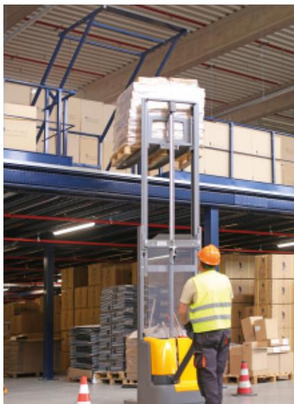
This installation houses Puccini's vast product range. Taking into account the limited space and type of goods to be stored, the company decided to instal a mezzanine floor that would double the useful storage area. To manage the goods, Mecalux fitted out the mezzanine floor with M7 heavy-duty shelving.
