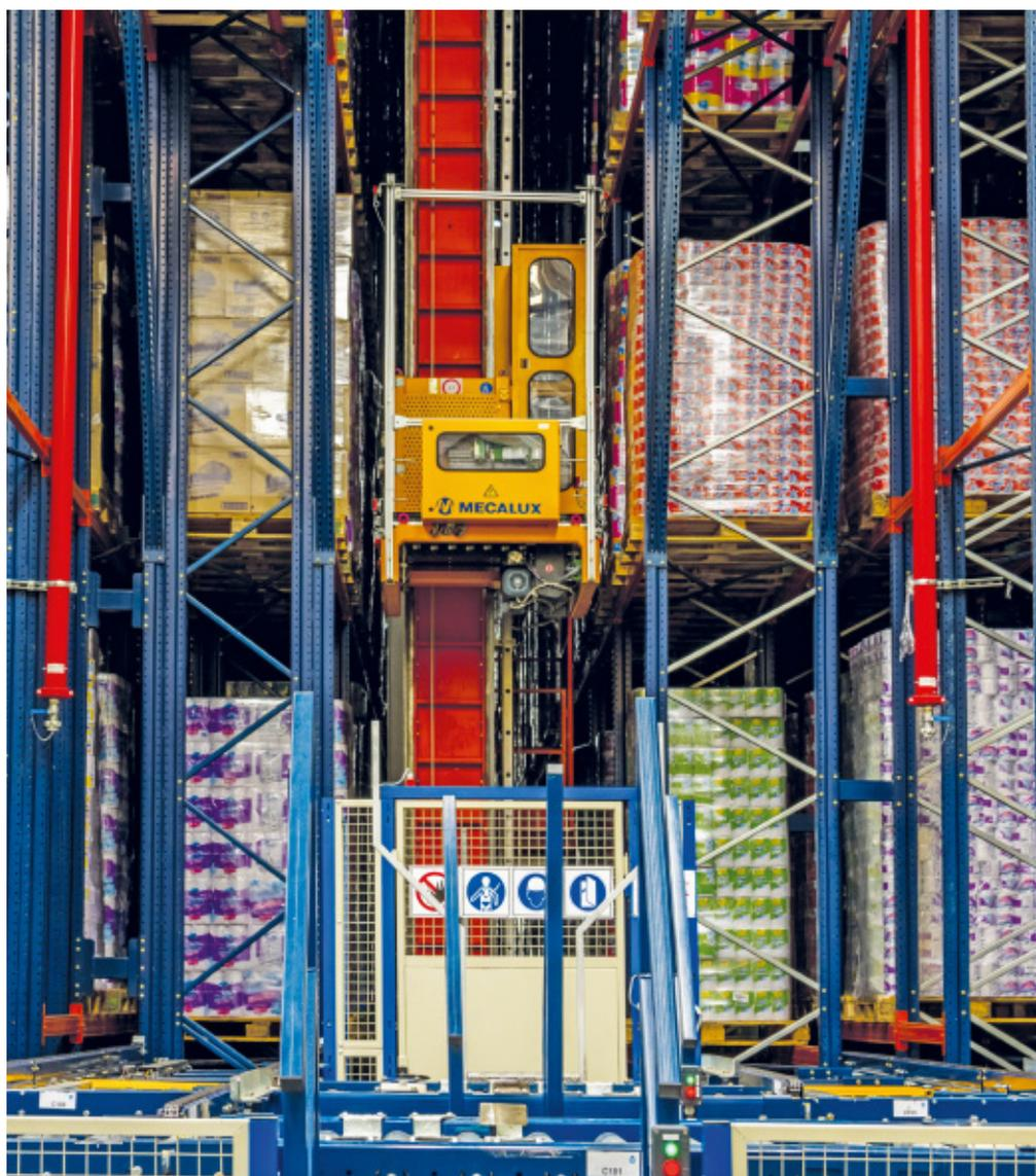
The installed automatic equipment ensure a high flow of goods per hour, to locate and remove pallets from the racking very quickly and without mistakes
