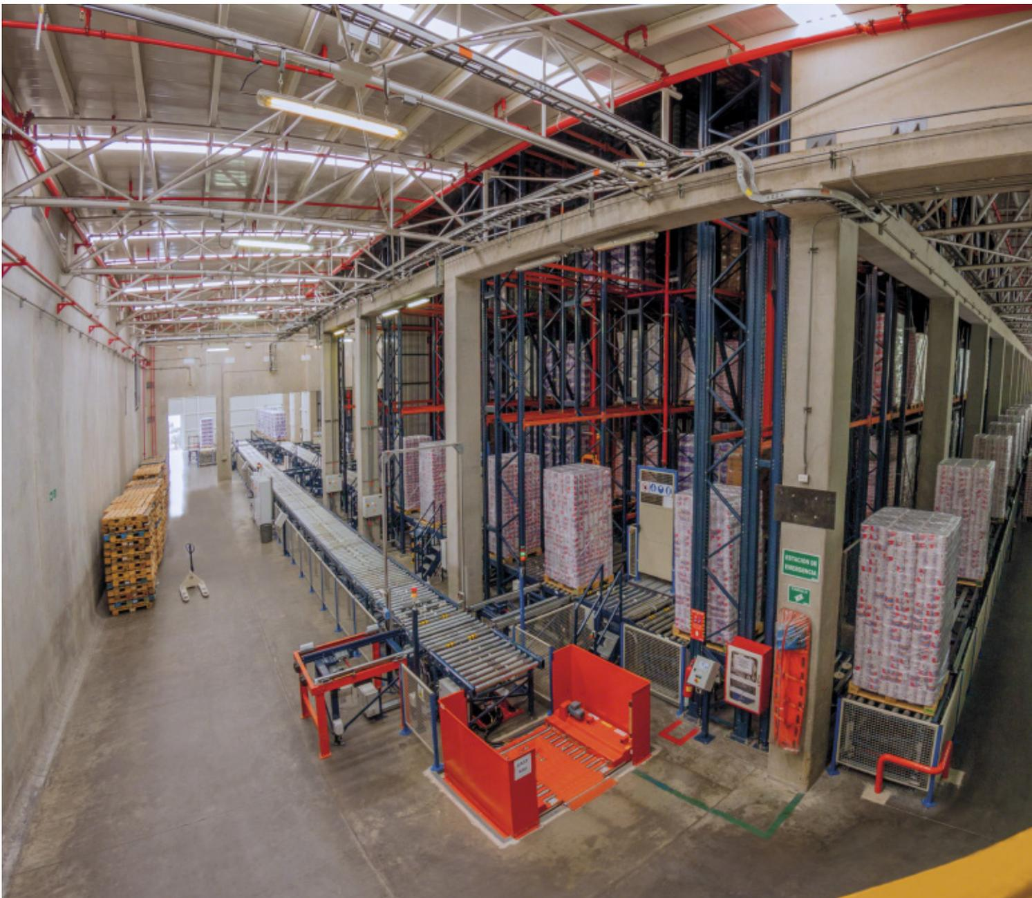
The recirculating conveyor circuit (double circuit) allows the management of inputs coming from production and from outside, as well as direct dispatches of palletised goods from the warehouse
