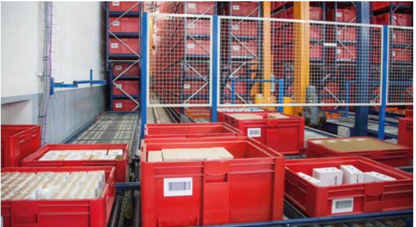
A twin-mast stacker crane circulates in each aisle with double forks in its cradle for 800 x 600 mm boxes.
