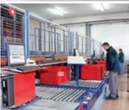
**Unidroco, wholesale leader in drugstore and perfumery items specialised in distribution, has an 800 x 600 mm automated miniload warehouse in their Barcelona logistics centre with capacity for more than 14,200 boxes. The installation is set up to automatically carry out product replenishment, all without interrupting order preparation. It is controlled by the Easy WMS warehouse management system by Mecalux.**
