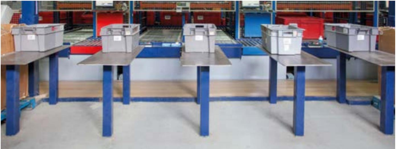
The front of the Unidroco automated warehouse has four picking stations equipped with put-to-light devices
