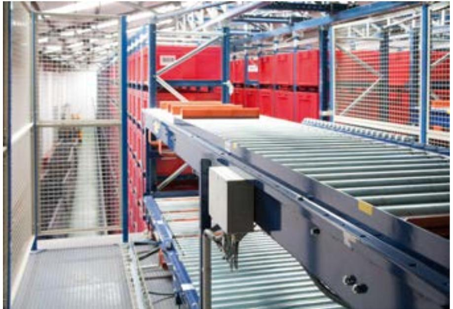
Mecalux supplied an automated miniload warehouse with a capacity for more than 14,200 boxes and a two-level conveyor: the lower for picking and the upper for replenishment
