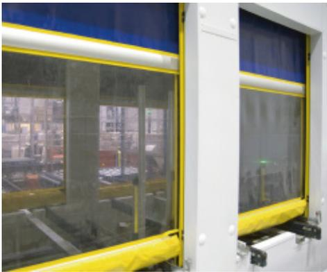
The input system protects the cold storage from sudden changes in temperature and pressure by the continuous flow of load units
