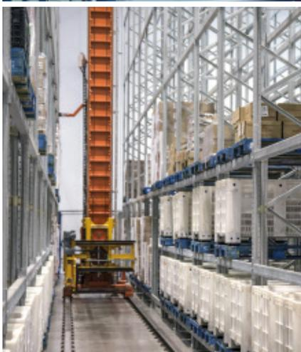
La Anónima, one of the most important supermarket chains in Argentina, has expanded its cold storage in the town of Ituzaingo (Buenos Aires), gaining greater storage capacity. Mecalux has installed an automated warehouse composed of four single-depth aisles served by trilateral stacker cranes and a conveyor circuit at the front; all managed by the warehouse management software the Easy WMS by Mecalux. This solution is designed to meet growing demand, adapting to future prospects.
