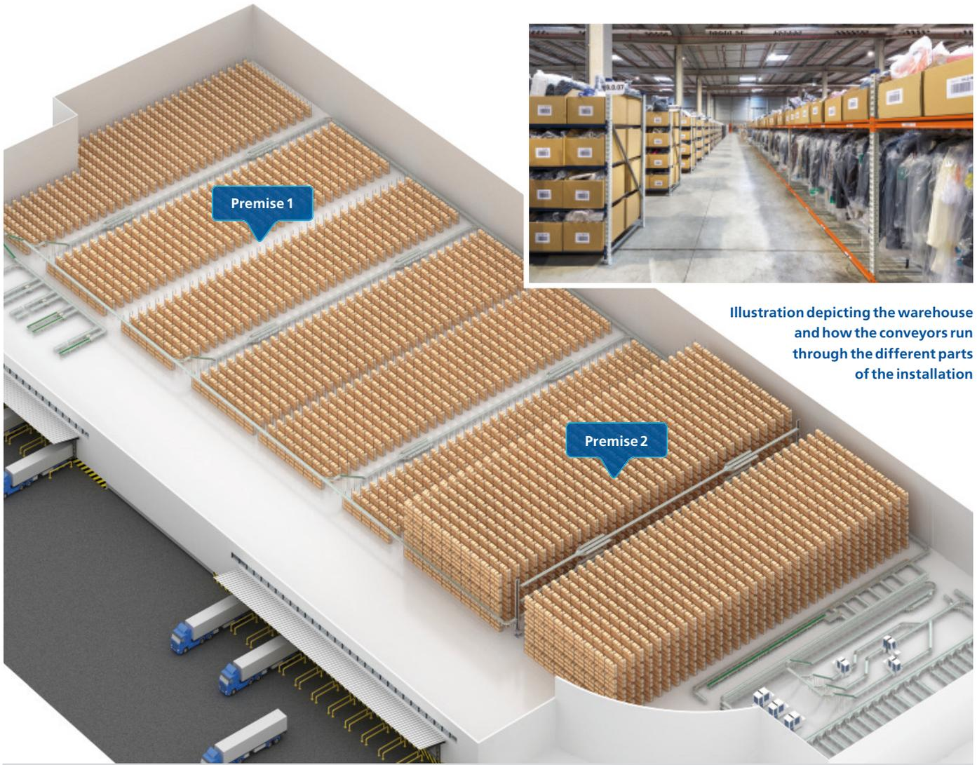
Illustration depicting the warehouse and how the conveyors run through the different parts of the installation
