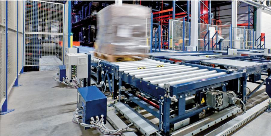
WOK, one of the most well-known packaging companies in Poland, has constructed a new automated clad-rack warehouse with a capacity for more than 6,300 pallets. It is equipped with stacker cranes adapted to the features of the installation and the products stored: they have telescopic forks that can handle up to four pallets deep per aisle side. Its operation is very fast and simple, controlled at all times by the Easy WMS warehouse management software by Mecalux.
