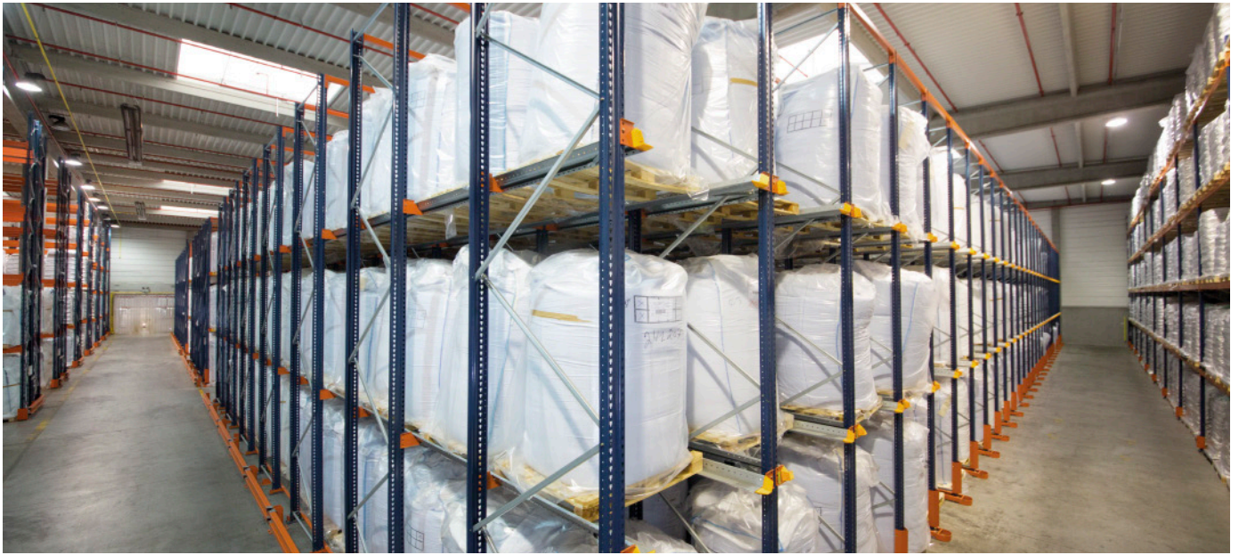
Drive-in pallet racking in the centre and conventional racking on both sides of the aisle
