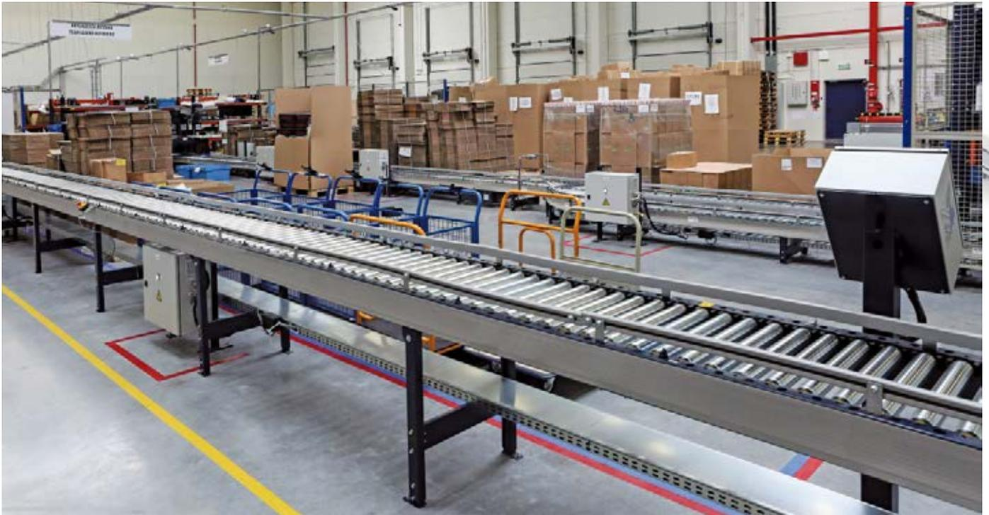
Boxes arrive to the picking stations via a conveyor circuit, which measures over 38 m long
