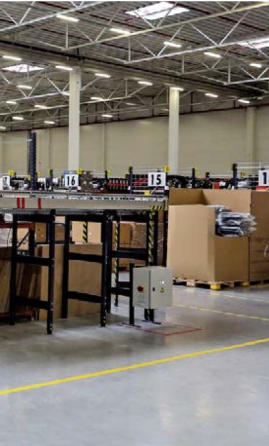
When the order is consolidated and the shipping box packed, it is introduced onto the intermediate level of the conveyor circuit and transferred to the sorting area, where it will be grouped by routes and agencies.
