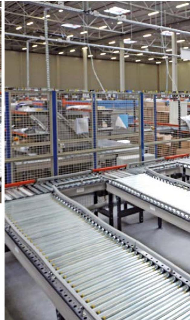
Conveyor ramps are on a 4% incline, allowing gravity displacement of the boxes
