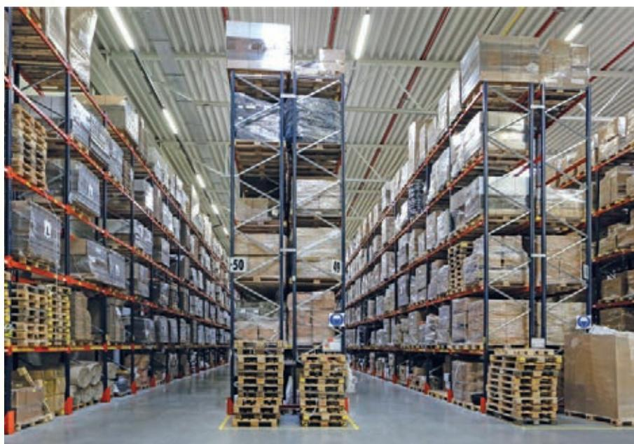
The racks have six load levels, with capacity to store over 5,000 pallets of 800 x 1,200 x 1,400 mm and a maximum weight of 920 kg
