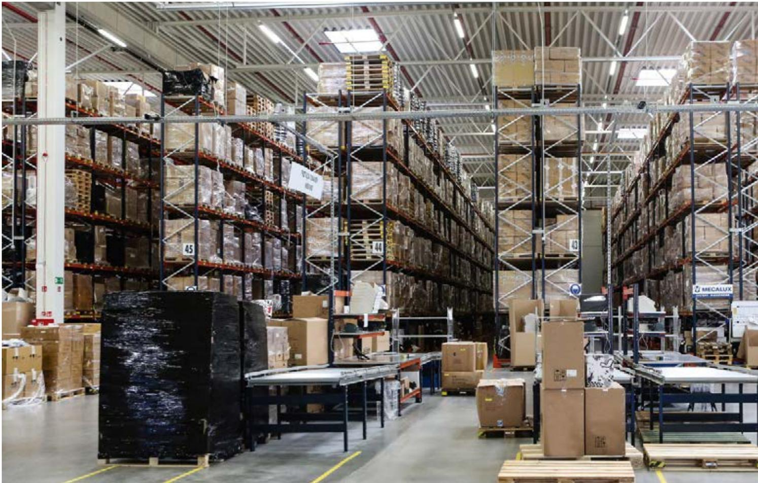
Eight conveyors receive goods from loading docks and four conveyors are dedicated to outputs of bulky products stored in pallet racking
