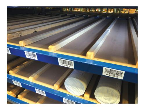
Rectangular, wooden laths serve to present shelves from bending and separate the fabric rolls stored in the racks
