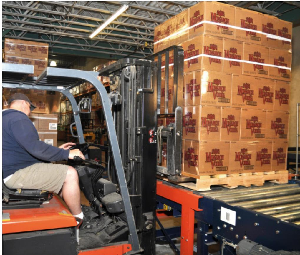
A secondary output station is located on the mezzanine level servicing split-case picking. When a stacker crane delivers a pallet to this station, a worker is given instructions on a computer screen to pick a required number of cartons. The cartons are removed from the pallet, labeled and placed onto the split-case conveyor supplied by IKML. Once the required box-
