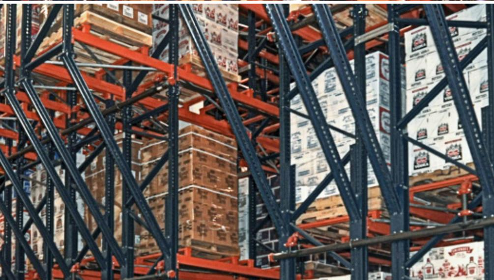
The newly installed pallet racking with stacker cranes supplied high-density storage in an even smaller footprint with room for many years of growth. The new AR/RS fully utilizes the 15.5 m high warehouse addition by adding nearly 2,800 more storage locations.
