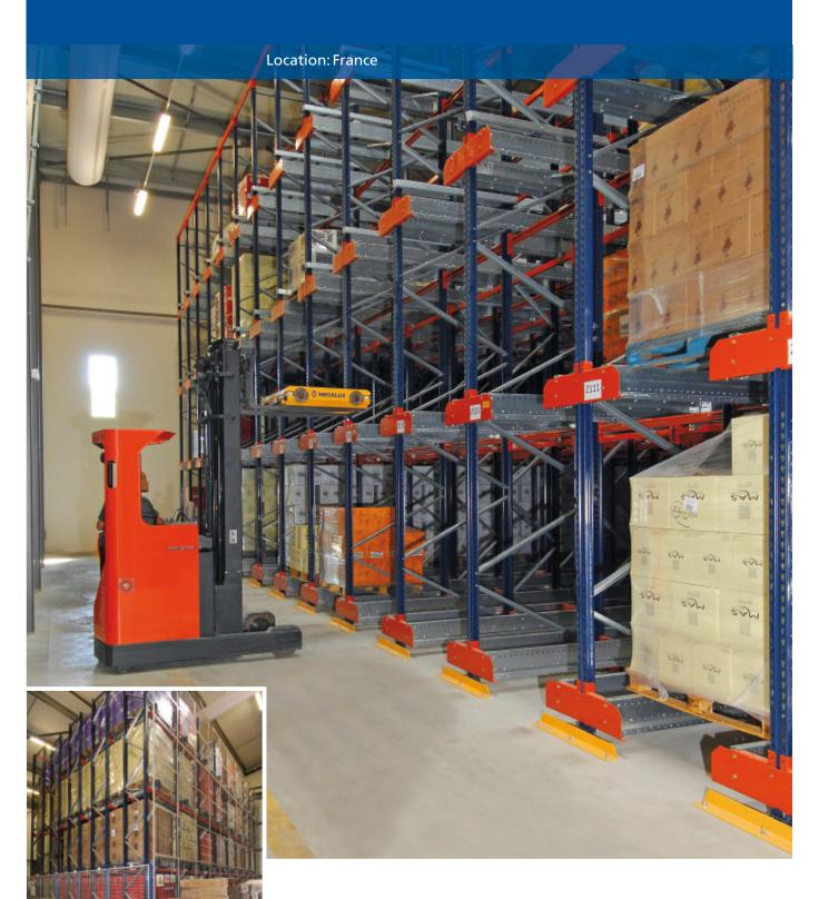
Mecalux reorganises the warehouse of the wine producer Domaines Paul Mas, divides it into three sectors and installs different storage solutions that fit the characteristics and operation of each product. Automation arrives in the form of the racking served by shuttles controlled by a Wi-Fi tablet and an automated vertical warehouse.
