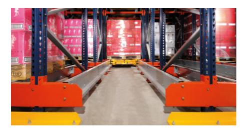
In addition, Mecalux offers the possibility of installing a positioning camera in the shuttle for the operator to view from the same tablet where and what the shuttle is doing at all times. Once the shuttle's battery runs out, the shuttle is automatically sent to the front of the channel, and the control tablet immediately notifies the operator that the battery is depleted. That is when it is moved to the battery charging station, set up to charge two shuttles at once.
